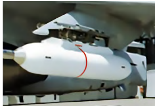
AIM-9X CTU on wing pylon
