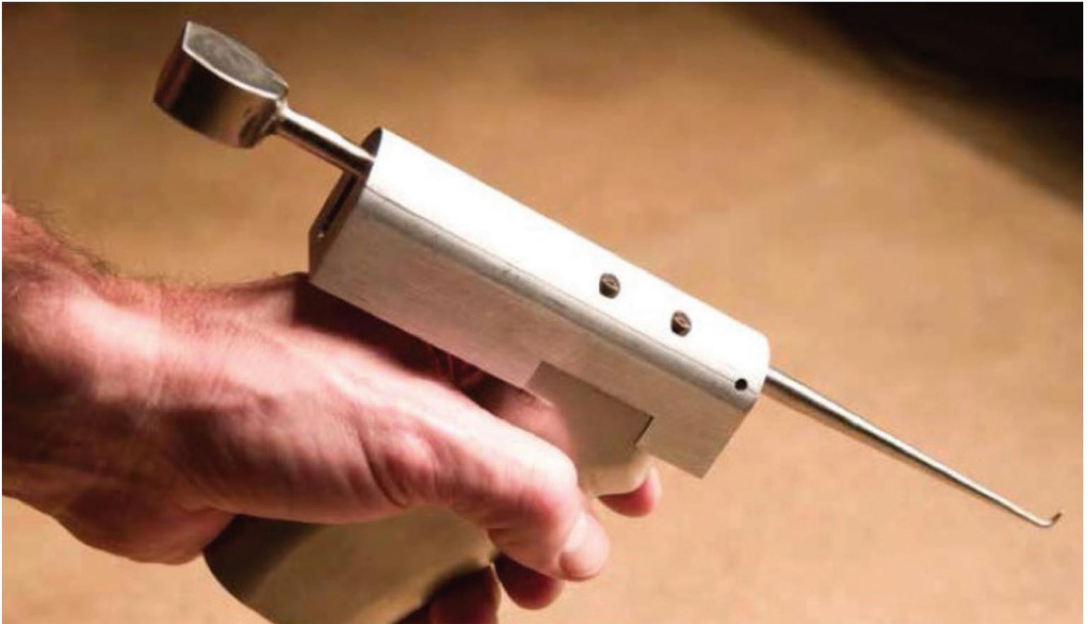
Microfracture awl that reduces unintended cartilage damage. Hinged handle allows for the physician to more easily deliver the force of the pick into the area of interest rather than laterally.
